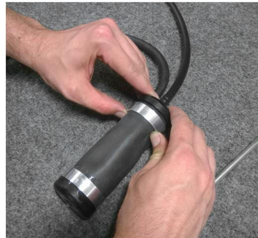
Slide Retention rings toward end of bladder, making sure bladder is centered
