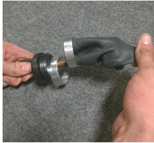
Pull bladder to be removed towards center, releasing retention rings.
