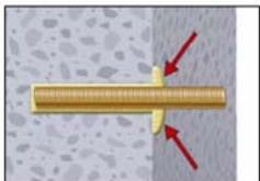
8. Be sure that the anchor is fully seated at the bottom of the hole and that excess mortar is visible at the top of the hole. If these requirements are not maintained, the application has to be renewed. For overhead installation fix embedded part (e.g. wedges).
