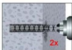
2b. Check brush diameter acc. Table 5 and attach the brush to a drilling machine or a battery screwdriver. Brush the hole with an appropriate sized wire brush  $> d_{b,min}$  (Table 5) a minimum of two times.
