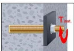
10. After full curing, the add-on part can be installed with the max. torque (Table 2) by using a calibrated torque wrench.
