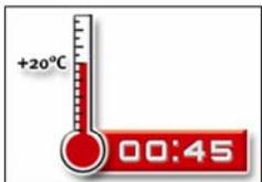
9. Allow the adhesive to cure to the specified time prior to applying any load or torque. Do not move or load the anchor until it is fully cured (attend Table 4).
