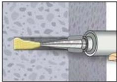
6. Starting from the bottom or back of the cleaned anchor hole fill the hole up to approximately two-thirds with adhesive. Slowly withdraw the static mixing nozzle as the hole fills to avoid creating air pockets. For embedment larger than 190 mm an extension nozzle shall be used. For overhead and horizontal installation in bore holes larger than  $\varnothing$  20 mm a piston plug and extension nozzle (Annex 8) shall be used. Observe the gel-/ working times given in Table 4.
