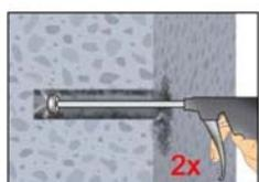
2f. Finally blow the hole clean again with compressed air acc. Annex 8 (min. 6 bar) a minimum of two times. If the bore hole ground is not reached an extension shall be used.
