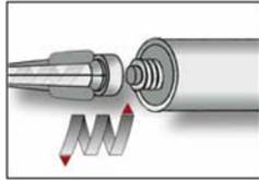
3. Attach a supplied static-mixing nozzle to the cartridge and load the cartridge into the correct dispensing tool.
