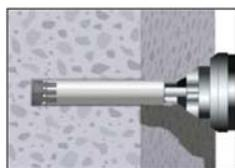
1b. Drill with diamond drill a hole into the base material to the size and embedment depth required by the selected anchor (Table 2 or Table 3).
