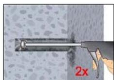
2d. Starting from the bottom or back of the bore hole, blow the hole clean with compressed air (Annex 8) (min. 6 bar) a minimum of two times. If the bore hole ground is not reached an extension shall be used.
