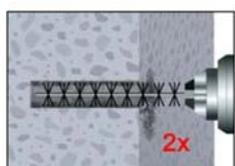
2e. Check brush diameter acc. Table 5 and attach the brush to a drilling machine or a battery screwdriver. Brush the hole with an appropriate sized wire brush  $> d_{b,min}$  (Table 5) a minimum of two times.
