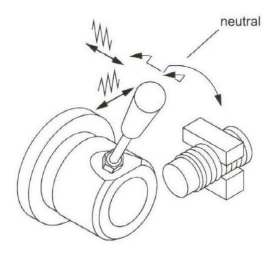
The apron handle is pushed to the front of the limit position, lift the black bakelite handle and counterclockwise rotate the handle to the limit position, realized cross feed cutting movement.
