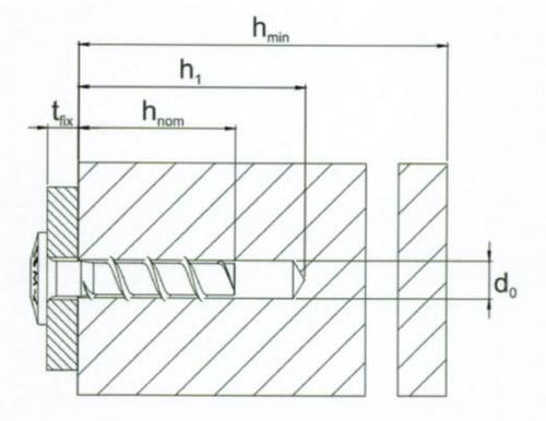
$\begin{array}{lll} h_{\text{nom}} & = & \text{nominal anchorage depth} \\ h_1 & = & \text{depth of the drill hole} \\ h_{\text{min}} & = & \text{thickness of member} \\ t_{\text{fix}} & = & \text{thickness of fixture} \end{array}$
