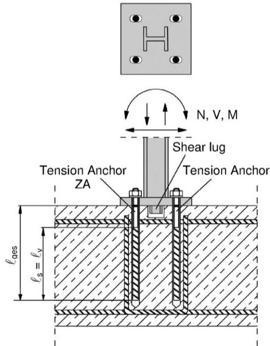
**Figure A7:** Overlap joint for the anchorage of barrier posts
