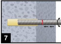
7. Push the reinforcing bar into the anchor hole while turning slightly to ensure positive distribution of the adhesive until the embedment depth is reached.
