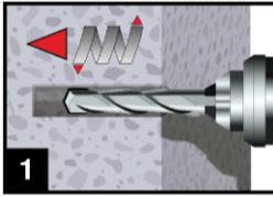
1. Drill a hole into the base material to the size and embedment depth required by the selected reinforcing bar with carbide hammer drill (HD) or a compressed air drill (CD). In case of aborted drill hole: the drill hole shall be filled with mortar.
