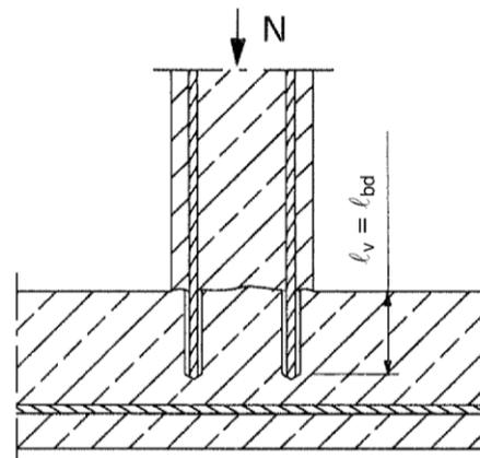
**Figure A5:** Anchoring of reinforcement to cover the line of acting tensile force
