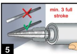
5. Prior to dispensing into the anchor hole, squeeze out separately the mortar until it shows a consistent grey colour, but a minimum of three full strokes, and discard non-uniformly mixed adhesive components.
