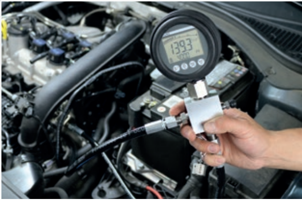
Dynamic testing with digital manometer, while the engine is running.
