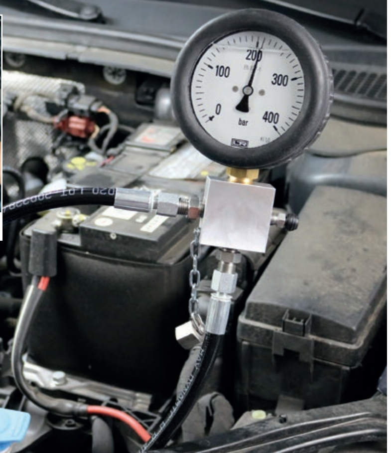
Dynamic testing with digital manometer, while the engine is running.
