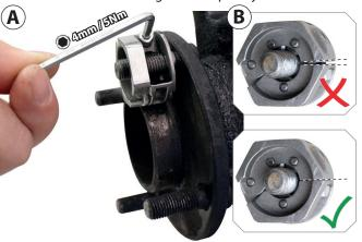
**13-4:** Lightly oil the damaged thread and reshape it.
