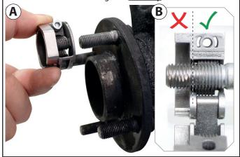
**3:** Close the re-threading tool completely.
