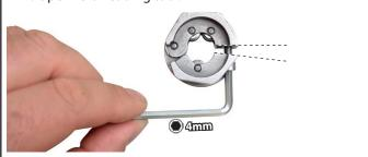
**2:** Place the re-threading tool <u>correctly</u> on the thread.
