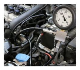
Before removing the high-pressure tester, the residual pressure must be released via the vent screw. To do this, connect the collection container to the vent screw, slowly open the vent screw and release the residual pressure, then loosen the flexible pressure line(s) from the pump and remove the tester.
