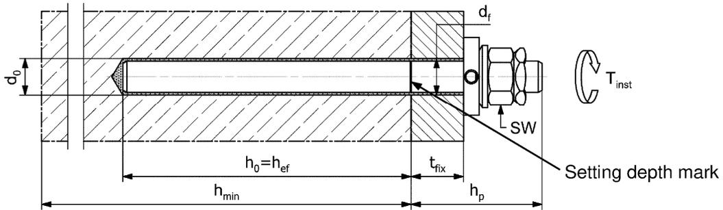
Installation conditions FIS A or RG M with washer
