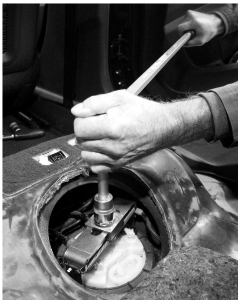
Abb. 4 : Loosening/Tightening the fuel tank sender lock ring.
