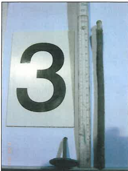
Photo 3: F10M202; dowel 1.3 load: 350N ; failure time: 140min
