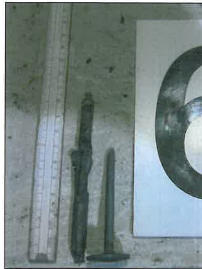
Photo 2: F8M132; dowel 2.6 load: 350N ; failure time: 82 min
