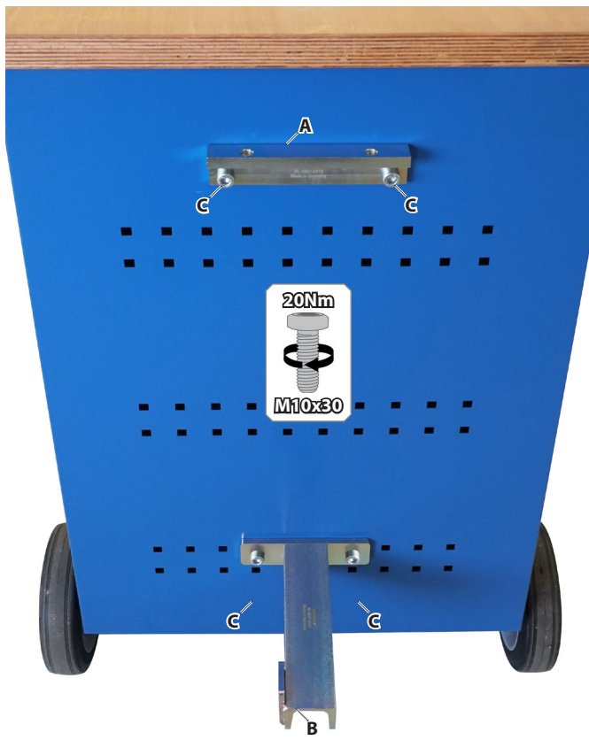
📷 2: Mounting the spring compressor - KL-5501 B on the wall bracket.
