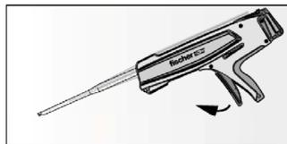
After injecting, release the dispenser. This will prevent further mortar discharge from static mixer.
