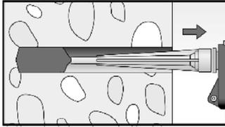
Inject the mortar from the back of the hole towards the front and slowly withdraw the static mixer step by step with each trigger pull. Avoid bubbles. Fill holes approximately 2/3 full, to ensure that the annular gap between the rebar and the concrete will be completely filled with adhesive over the entire embedment length. The conditions for mortar injection without extension tube can be found in **Table B5.3**.
