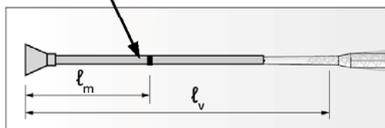
Mark the required mortar level  $l_m$  and embedment depth  $l_v$  resp.  $l_{e,ges}$  with tape or marker on the injection extension tube.
