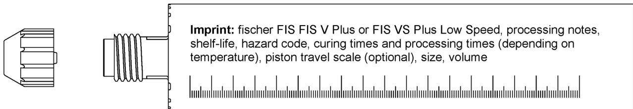
**Static mixer FIS MR Plus for injection cartridges up to 410 ml**
