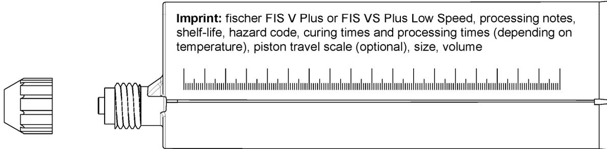
**Injection cartridge (coaxial cartridge) FIS V Plus with sealing cap; Sizes: 300 ml, 380 ml, 400 ml, 410 ml**
