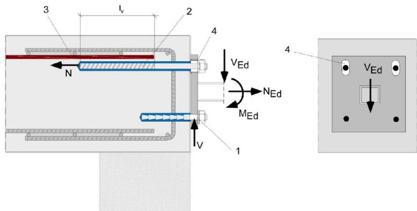
The required transverse reinforcement acc. to EN 1992-1-1:2011 is not shown in the figures. **The fischer rebar anchor FRA may be only used for axial tensile force.** The tensile force must be transferred by lap to the existing reinforcement of the building. The transfer of the shear force has to be ensured by suitable measure, e.g. by means of shear force or anchors with European Technical Assessment (ETA).
